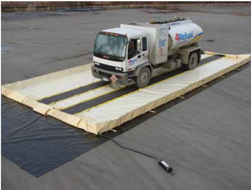
TOP Operators need to have plans for fuel containment. SEI Photo
